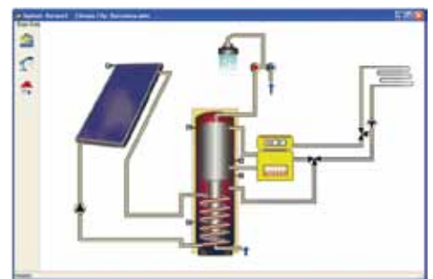
Example of a System Configuration in T*SOL®
